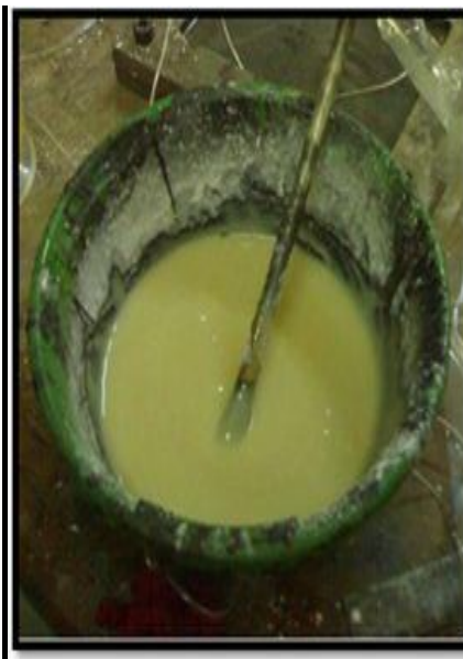
Fig 3. Mixture of Resin, Hardener and Filler
